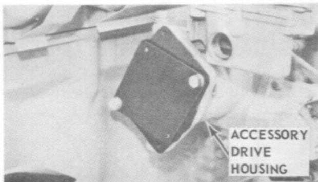
TIMING FIXTURE PLATE INSTALLED
